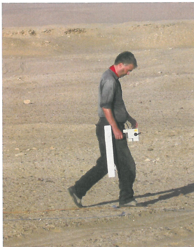
The FM256 Gradiometer in action
