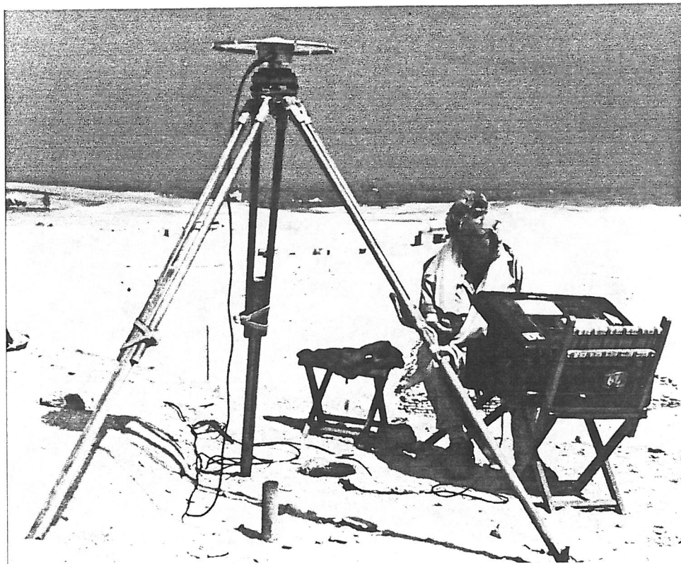
Ashtech Z-12 GPS Receiver on Unas Pyramid (a.)
