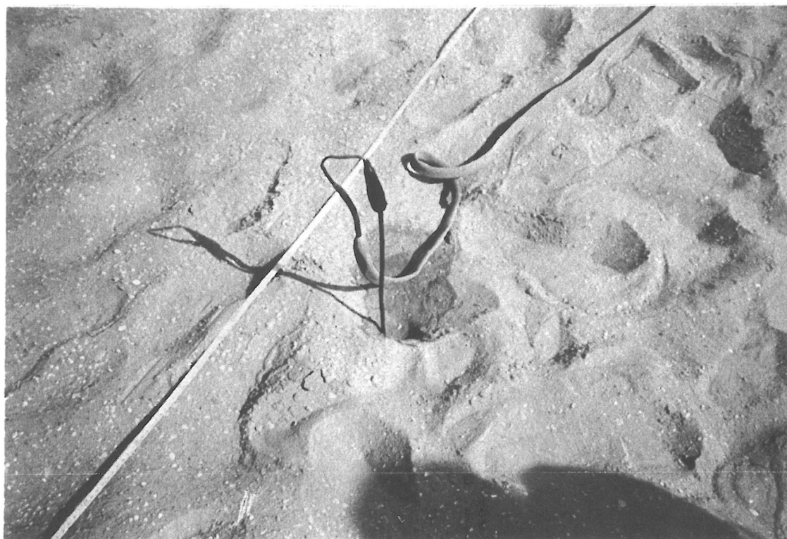
Copper Electrode in Position
